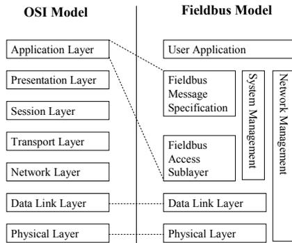
**Figure 2: Foundation Fieldbus Standard**
